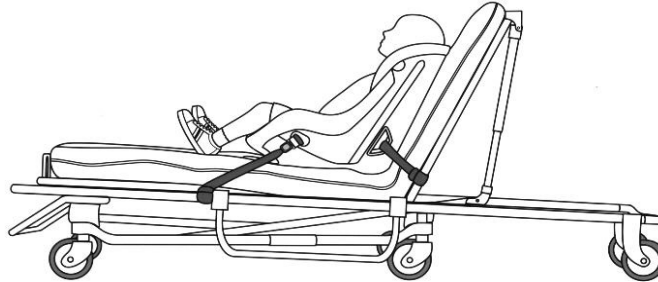
Figure 4. Recommended method for restraining children up to about 18 kg who can tolerate a semi-upright seated position, showing belt attachment to the cot and routing through the convertible child restraint.
