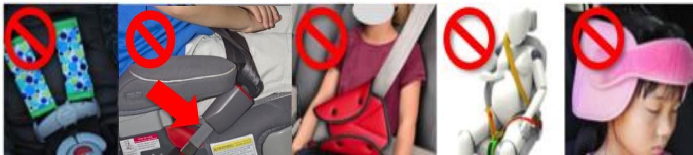
Products such as belt extenders, belt adjusters, covers, and head restraints can alter the way that safety belts and safety seats work, reducing protection in a crash.
